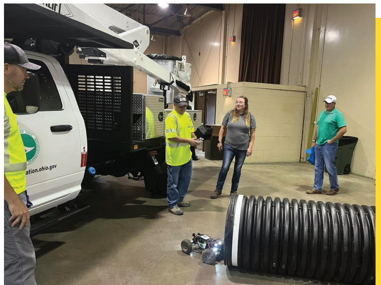
ODOT employees test the HIVE vehicle through a makeshift culvert.
