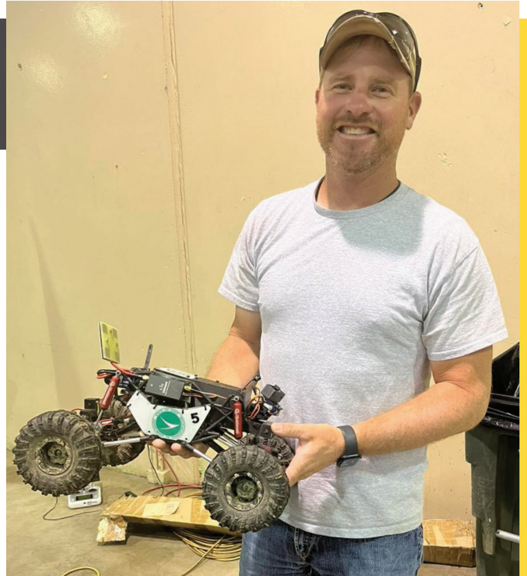
Davey Christman, ODOT Dist. 10, shows off the HIVE, a motorized truck with a camera that finds obstructions workers can't always see.
